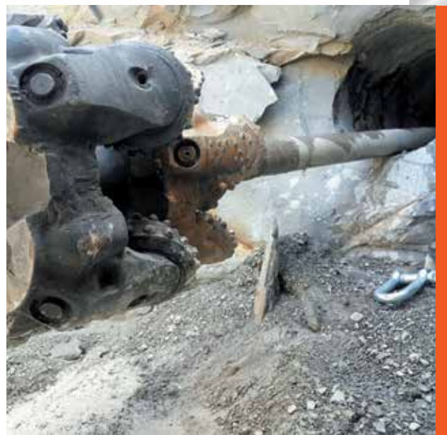
IV stage of drilling: on a shaft set a Rolling Cutter disk of Ø 500 mm. and Ø 600 mm.
